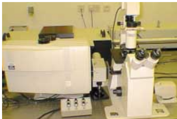
Fig 4 (right) The position of the external detector unit, and electronics control unit, in relation to a typical Bio-Rad multi-photon system, in this case an MRC-1024MP installed on a Zeiss inverted microscope. Other configurations are also available.
