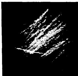
Fig. 5. Picture of 20% sodium oleate jelly; solidified slowly (at approx. 10^{\circ} ). Apochromat 3, ocular 1, magnification 140. Cardioid condenser (Siedentopf).
