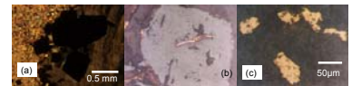
Fig. 3: Textural relations in Egat: (a) pseudomorphs of goethite after pyrite next of wall rock selvages. (b) Stringers of Au in goethite after Py/Asp; polarized reflected light, 320µm across. (c) Au specks in chlorite from the alteration zone.
